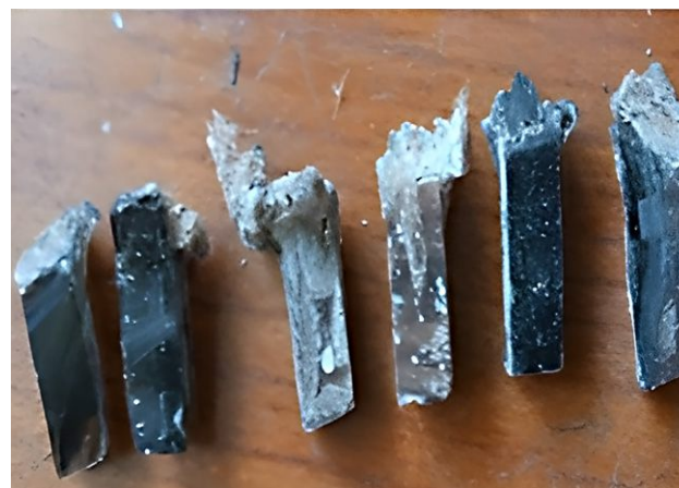
Figure 11. Test samples of carbon/sisal composites after testing
