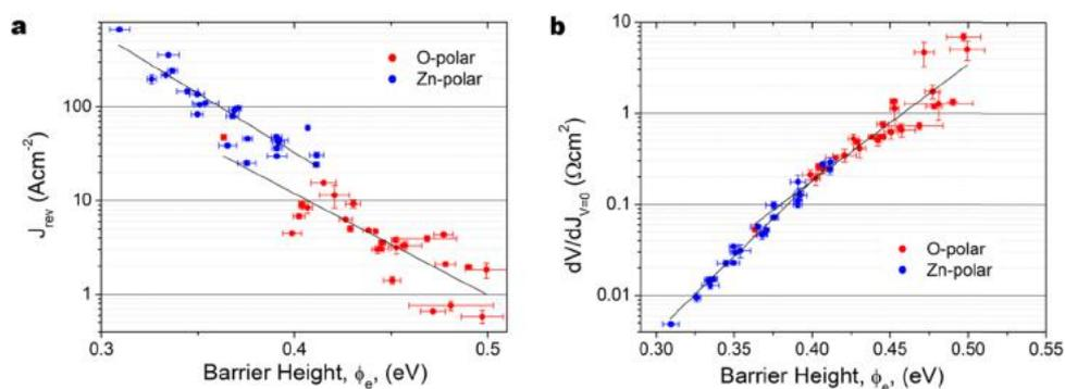
**Figure 3.** (a) Graph showing the average current density for each nanorod at  $-2$  V reverse bias plotted against  $\phi_e$  and showing exponential functions fitted to each data set. (b) Graph showing the relationship between the specific differential resistance for each of the O-polar and Zn-polar nanowires and the exponential fit to each data set.
