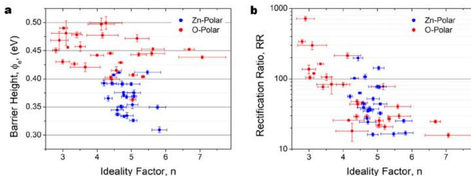
**Figure 2.** (a) Graph showing the relationship between ideality factor,  $n$ , and effective barrier potential height,  $\phi_e$ , for measured nanorods on the Zn-polar and O-polar samples after the oxygen plasma treatment. (b) Graph showing the rectification ratio of Zn-polar and O-polar nanorods with Au contacts plotted against the ideality factor.
