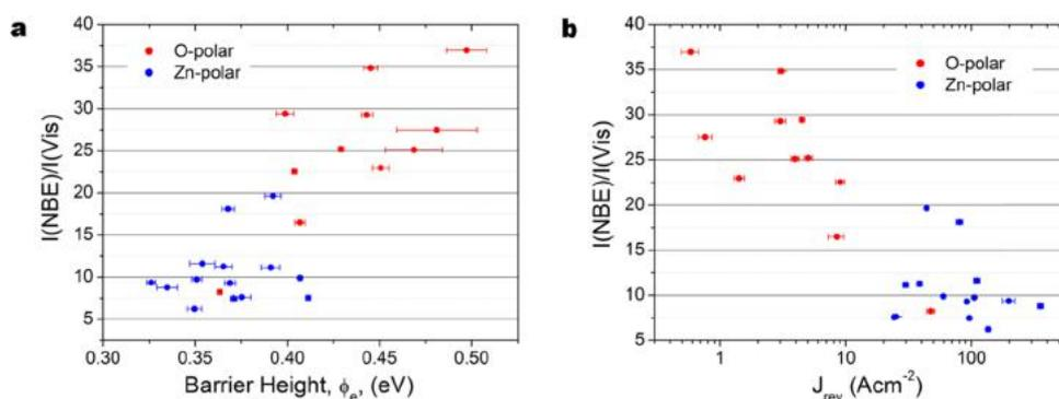
**Figure 5.** Graphs comparing the CL data for both samples with properties of the Au–ZnO contacts. (a) Intensity ratio of the NBE emission and visible band ( $I_R$ ) against barrier height ( $\phi_e$ ); (b) intensity ratio of the NBE emission and visible band ( $I_R$ ) against the current density at  $-2$  V ( $J_{rev}$ ).
