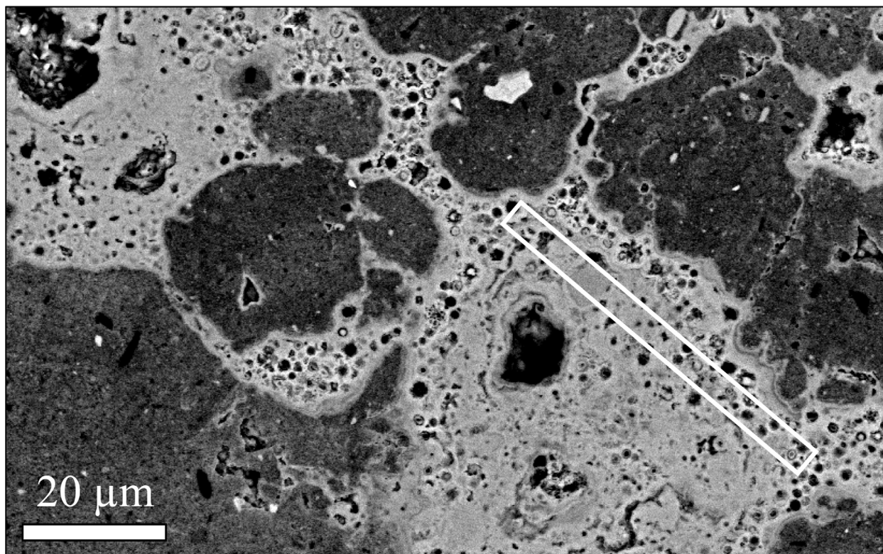
Figure 6. Backscattered scanning electron micrograph of encrusted cell envelopes that had infilled pore spaces between gibbsite-rich clasts. The rectangle highlights the regions from which a lamella was extracted using a focused ion beam scanning electron microscope for NanoSIMS analysis (refer to Figs. 7 and 8).
