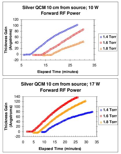
The graphs above show the results of tests with silver-coated QCMs using room air and performed at the three pressure and two power settings used in the gold-coated contaminated QCM tests. The thickness changes on the silver-coated QCMs are due to exposure to oxygen atoms and can be predicted by the Deal-Grove Model [4]. The Model can be used to determine the oxygen atom concentration at the QCM (10 cm from source). The table below shows the results of the tests using the silver-coated QCMs.
