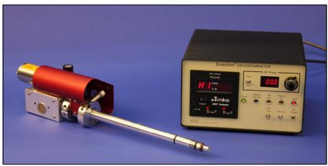
The picture above shows the remote plasma cleaner system using the TEM Holder. A shroud surrounding the valve assembly allows the user to manipulate the ORS on a TEM Holder more easily and provides a more aesthetic package.
