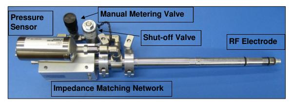
The picture above is of the Oxygen Radical Source (ORS) on a TEM Holder. The RF electrode is on the right hand side near where a TEM sample would normally be. The manual metering valve, shut-off valve, pressure sensor, and impedance matching network are on the left hand side of the picture and are outside the TEM chamber during operation of the ORS.
