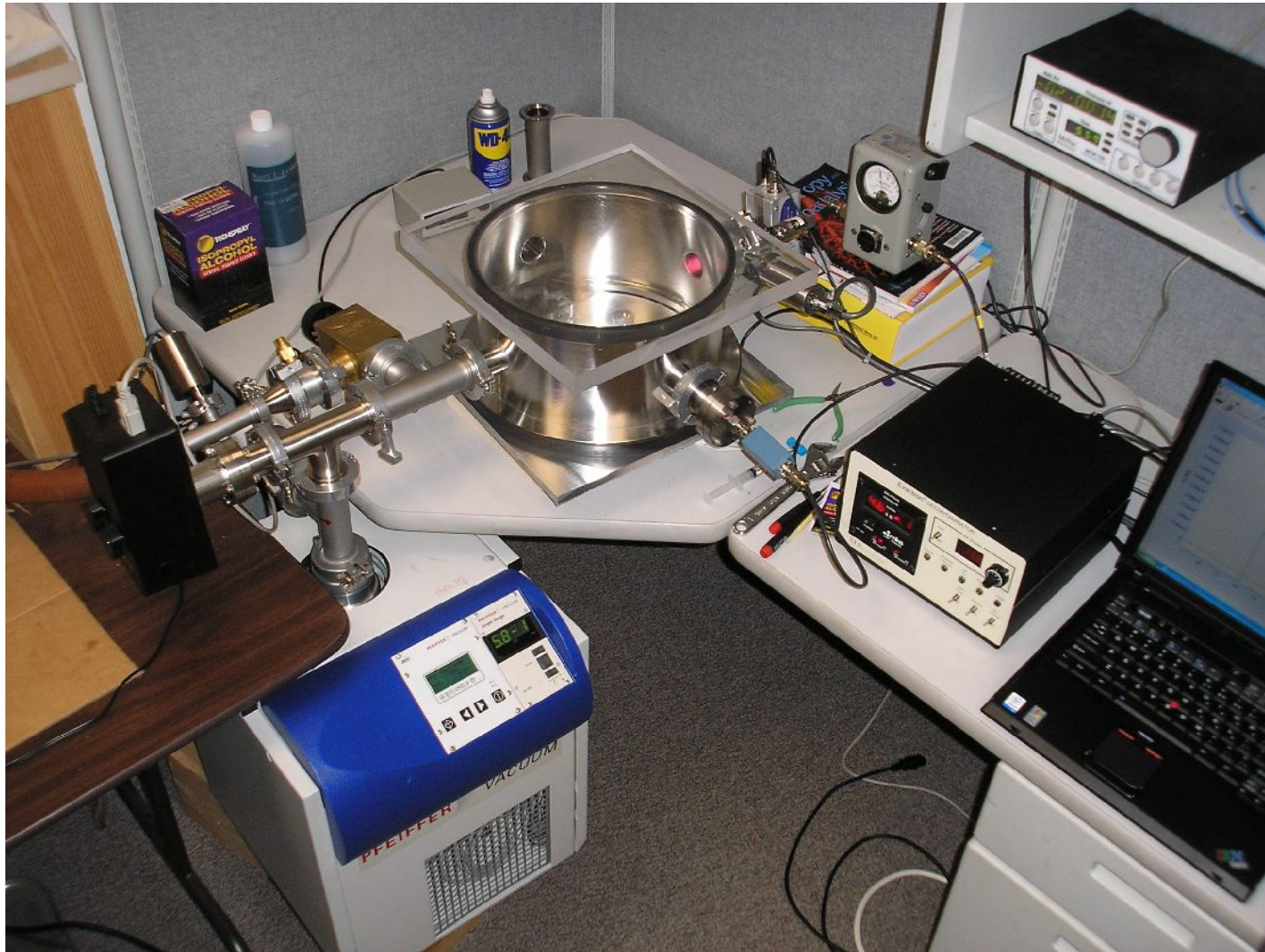
Figure 2 Evactron mounted on test chamber with RF power meter, RGA and quartz crystal monitor attached. Pink glow is Evactron plasma.
