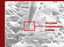
FIG. 3: Evactron cleaning experiment. Probe tip after 120 minutes under the SEM beam at 15,000X.
