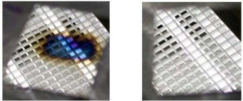
Previous tests of the Evactron De-Contaminator have shown that it can clean a silicon-capped EUV mirror such as the one above using room air without damage to the surface of the optic. The reflection seen on the optic is that of a fluorescent light on the ceiling above the optic. These pictures are courtesy of Patrick Naulleau of Lawrence Berkeley National Laboratory.
