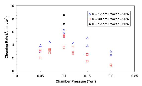
There is an increase in cleaning efficiency if the power goes from 20 to 30 W. We expect that this increase in cleaning efficiency will continue as the power delivered to the RF plasma increases. The RF generator can deliver up to 65 W of forward RF power.
