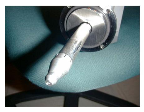
Figure 1: Oil condensed on EDS detector snout and collimator. Oil on EDS detector window adsorbs C X-rays and interferes with quantitative analysis. Evactron cleaning removes this oil without damage to the UTW window
